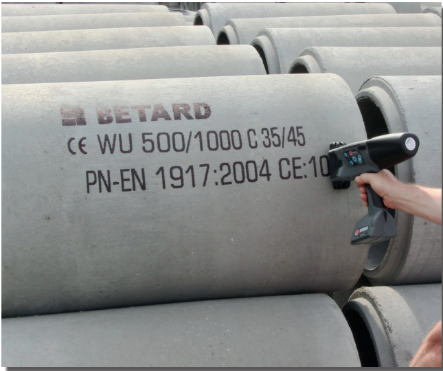
Prints on concrete with special UV-resistant black ink
