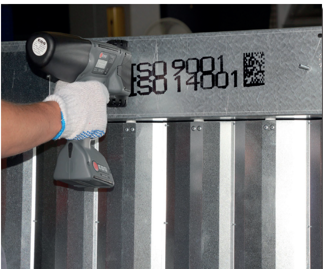
Prints on steel - 2D barcode - with black universal ink
