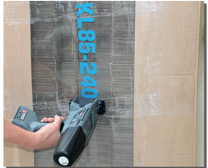
Prints on stretch wrap with pigmented ink
