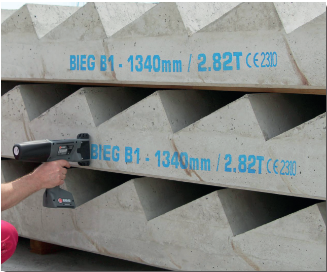
Prints on concrete with blue pigmented ink
